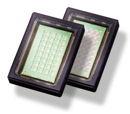
Snapshot mosaic hyperspectral image sensors with 16 and 25 bands channels - conceptual view of the per-pixel filter
